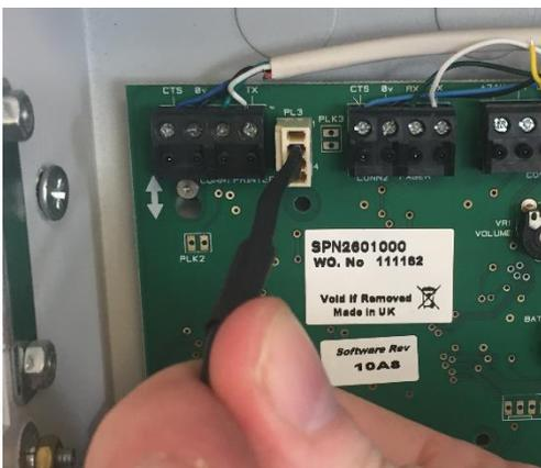
Programming connector on the Quantec panel
