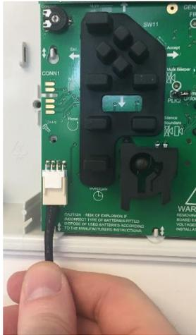
Programming connector on the 16 Zone XFP panel
